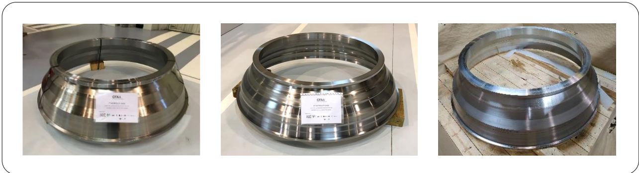
Figure 3. Three full scaled demonstrators manufactured by Near Net Shape in HUC project.
